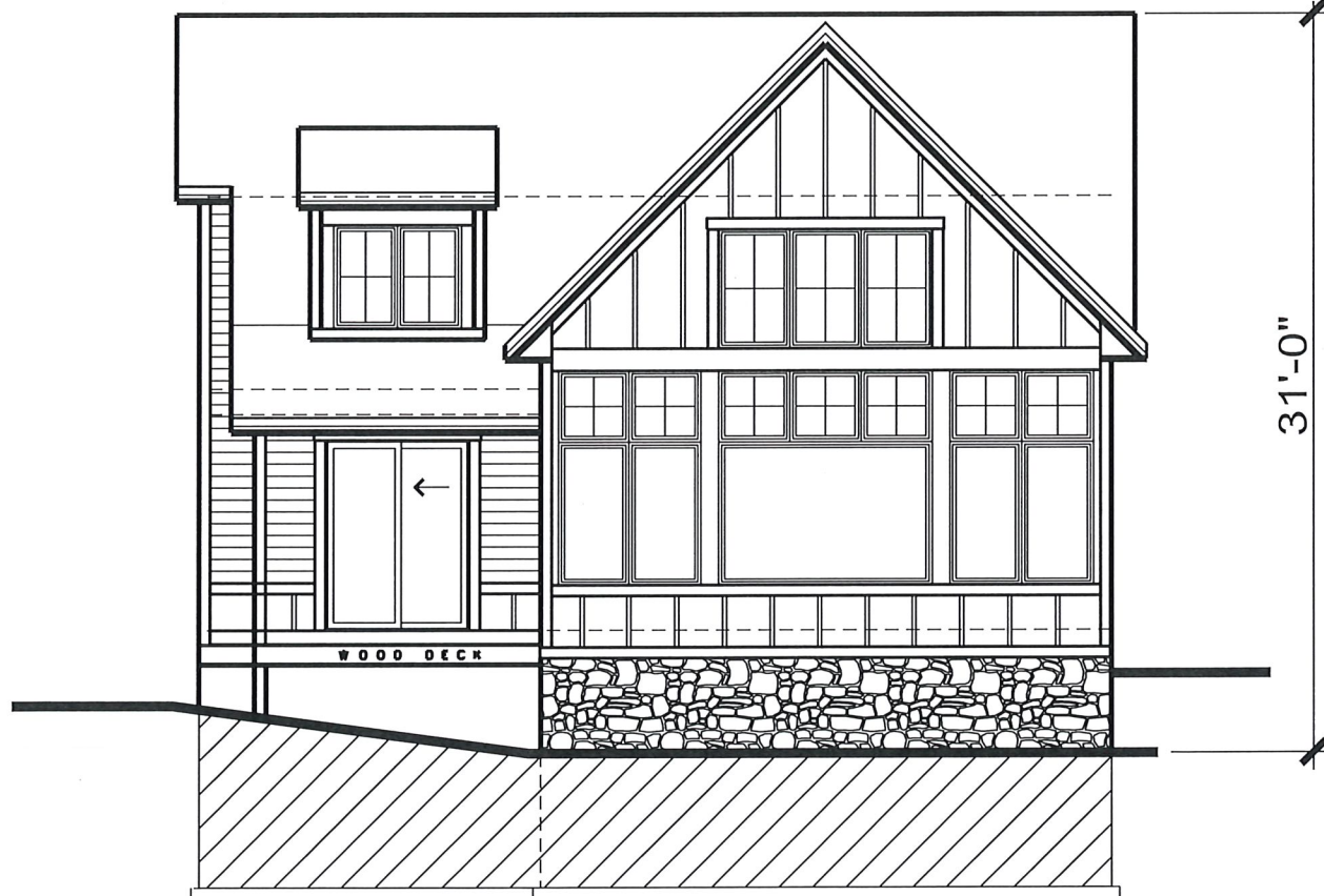
lakeside elevation 60% basement below grade
